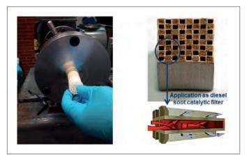
**Figure.** Ceramic filters developed to inactivate viruses in air samples.
